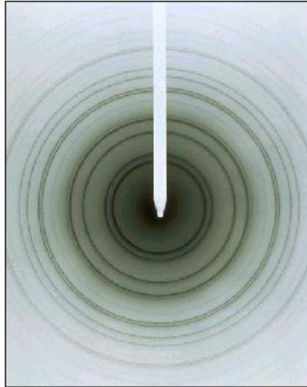
Electron diffraction through a sheet of crystalline aluminium (historic experiment)
